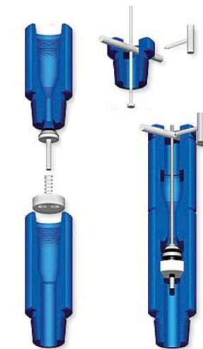
Inside Blowout Preventer
